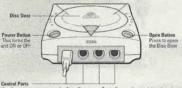
Use these ports to connect the Sega Dreamcast Controller or other peripheral equipment. From left to right are Control Port A, Control Port B, Control Port C, and Control Port D. Use each port to connect controllers for players 1 to 4 respectively.
